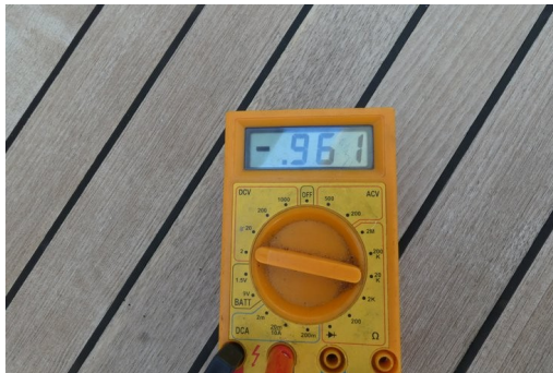
21. Test of cathodic protection on a 90' steel motor yacht: the unprotected steel potential is (see table aside) -600 to -710mV; the reading is -961mV, so the difference is in the range of 251~361mV, i.e the hull is correctly protected. The readings were taken in various locations around the vessel.
