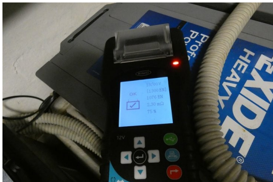
16. RBAG700 at work; this battery is at its 75%, with an IR of 2,3mΩ, so it's still good
